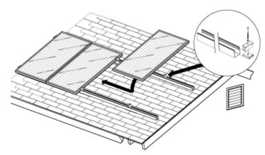
After the first module is secured, slide two intermodule clamp sets onto the first module side frame. They are designed to stay in place, freeing you up to slide and align the next module into place. Repeat this procedure until all modules are installed onto the support rail.
