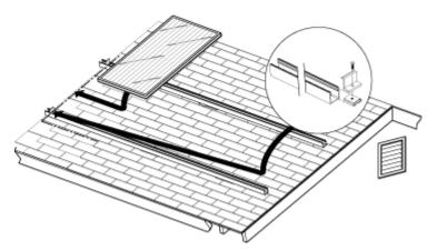
Slide the two end clamps near the end of the support rail and install your end module (first). Carefully square the module to the frame and tighten the clamps using a 1/2" box wrench or drive socket. **DO NOT OVER-TIGHTEN**, we recommend a maximum torque of 12 foot pounds to prevent damage to the module.
