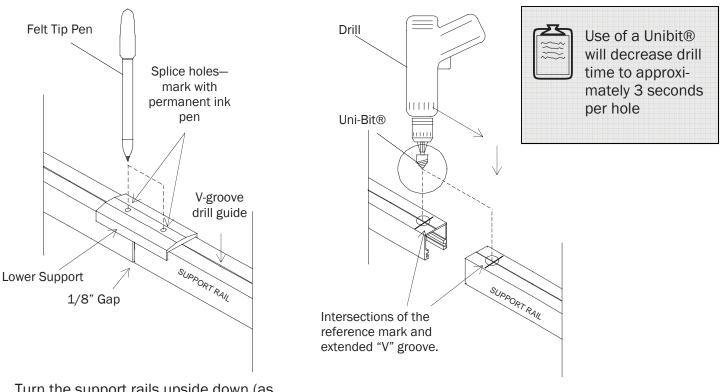
Turn the support rails upside down (as illustrated) so the bottom is facing up. Place the lower support over the rails to use as a template. Center the lower support over the rails and mark along the V-groove drill guide using a small felt pen.
