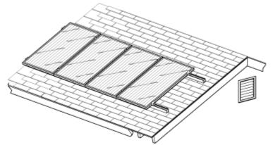
Upon installation of the last module in the panel, install the module end clamp to the end of the last module. Before fully tightening the bolts, make any adjustments needed to create a square and even array. Once all modules are in the position desired, use a 5/16" Socket impact set to 12 ft. Ibs to tighten the bolts on the clamps.
