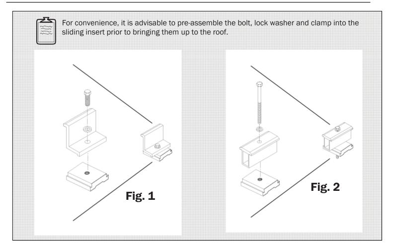
Attachment and clamping of the solar modules to TileTrac<sup>®</sup> or FastJack<sup>®</sup> attachments works exactly the same. After the support rails have been fastened, you are ready to install the solar modules. There are two sets of clamps; the outside clamps (end clamp) (Fig. 1) and the inter-module clamps (Fig. 2) that install between the modules.
