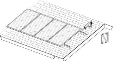
To complete the installation, cut off any excess support rail not used with a reciprocating saw. You may want to use an extrusion blade.
