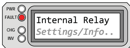
Figure 5-38, Internal Relay Fault
