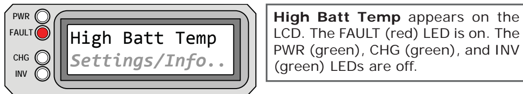
Figure 5-23, High Battery Temperature Fault
