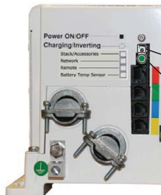
Figure 6-1, Performing an Inverter Reset
