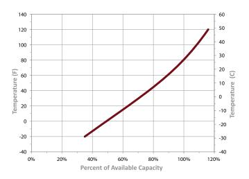
A. The amount of amp-hours (AH) a battery can deliver when discharged at a constant rate at 77°F (25°C) and maintain a voltage above 1.75 V/cell. Capacities are based on peak performance.
