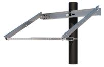
Side of Pole Mount is designed to fit pole diameters of 2" to 4", and to support modules with a center-center weight distribution sized from of 19" to 39". Tilt range includes 15 - 65 degrees. IronRidge Side of Pole Mounts are manufactured using heavy-duty corrosion-resistant 5052-H32 aluminum.
