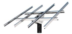
**Top Of Pole Mount** is a heavy duty mounting system ideal for single pole, multi panel arrays with a tilt range of 15 - 65 degrees. Mounted above either 4" or 6" poles, this configuration supports most manufacturer's modules. Our Top of Pole mounts are manufactured using powder coated steel and heavy-duty corrosion-resistant 5052-H32 aluminum.
