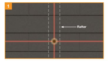
Locate rafters and snap vertical and horizontal lines to mark locations of flashings. Drill 1/4" pilot holes, then backfill with an approved sealant.
