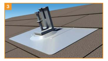
Line up pilot hole with flashing hole and insert lag bolt through bonded washer, L-Foot, and flashing. Tighten lag bolt until fully seated.
