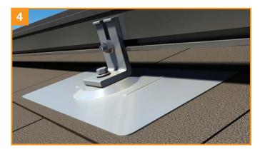
The FlashFoot is now installed and ready for IronRidge Rails. With provided L-foot fasteners preloaded into rails, drop rails into open L-foot slots.
