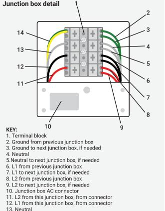
14. Ground from this junction box, from chassis screw
