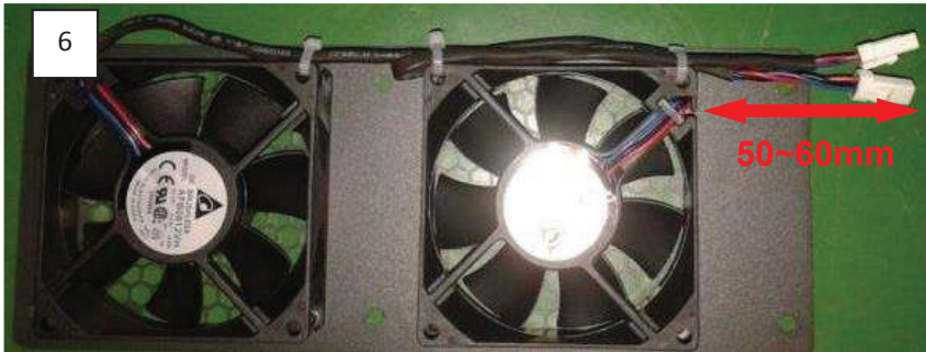
Figure 6.1 - Replace Cooling Fans
