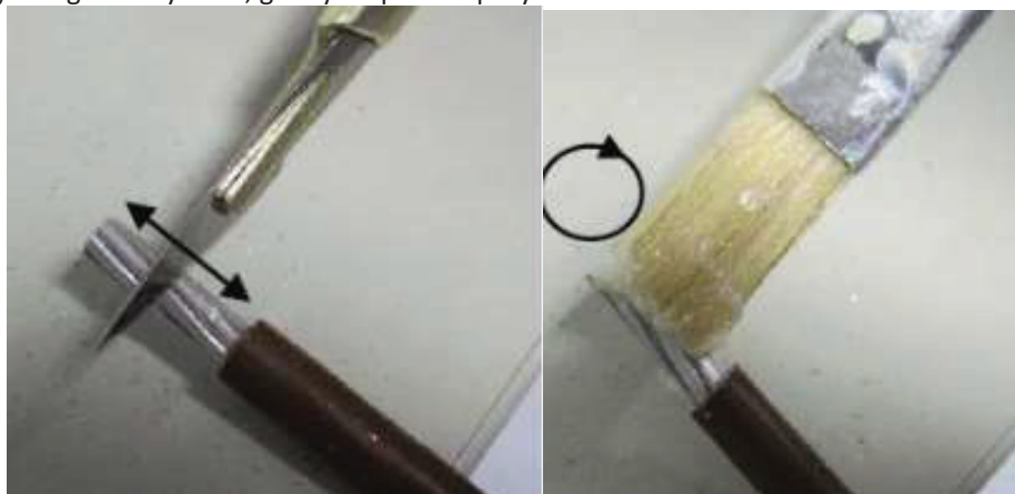
Figure 2-27 Preparing aluminum wires prior to connecting
