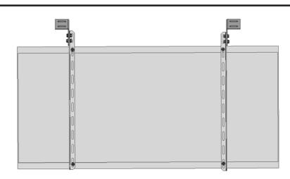
◆ If the distance between the PV module mounting holes is 26.9" or more, attach the clips to the rails so the protruding end of the clips are facing the center of the module.
