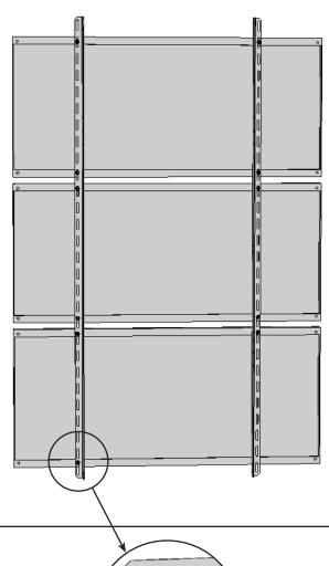
2. Secure the rails with a bolt, lock washer and hex nut in each of the PV mounting holes (4 on each panel).
