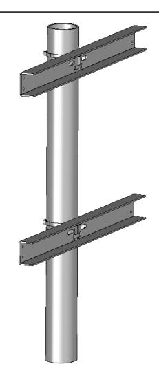
3. Once the hose clamps are in the desired position, tighten the hose clamp screws to 35 inch-lbs.
