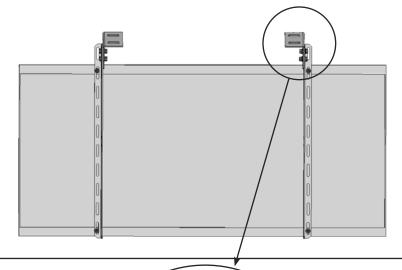
2. Attach the clips to the rails. In each of the mounting holes, use a bolt and flat washer on one side, and a flat washer, lock washer and nut on the other.
