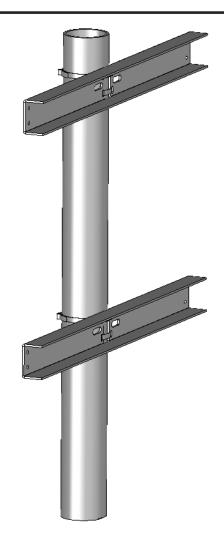
3. Once the hose clamps are in the desired position, tighten the hose clamp screws to 70 inch-lbs.
