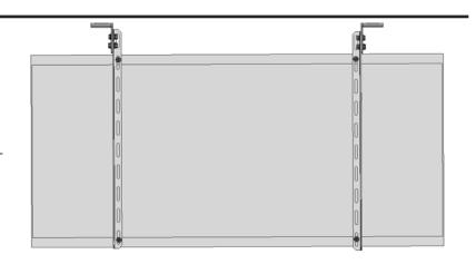
If the distance between the PV module mounting holes is 37 1/8" or more, attach the clips to the rails so the protruding end of the clips are facing the center of the module.
