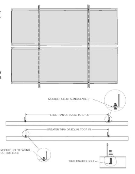
2. Secure the rails with a 1/4 - 20 x 3/4" bolt, lock washer and hex nut in each of the PV mounting holes (4 on each panel).
