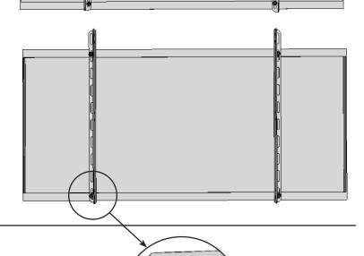
2. Secure the rails with a bolt, lock washer and hex nut in each of the 4 mounting holes.
