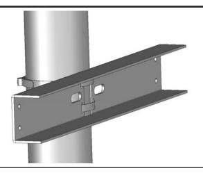
2. Tighten the hose clamp screws to 70 inchlbs
