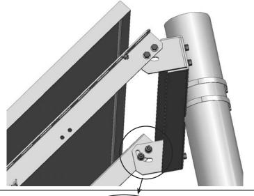
If desired, loosen the bolts holding the rails to the clips, and adjust the tilt of the panel as required
