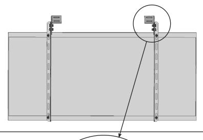
2. Attach the clips to the rails. In each of the mounting holes, use a bolt and flat washer on one side, and a flat washer, lock washer and nut on the other.
