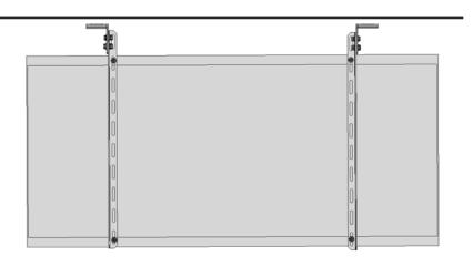
If the distance between the PV module mounting holes is 37 1/8" or more, attach the clips to the rails so the protruding end of the clips are facing the center of the module.
