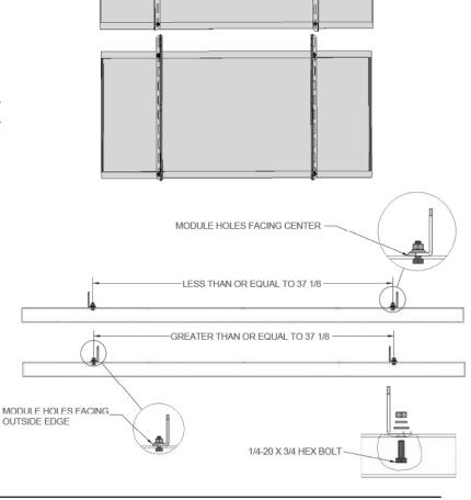
2. Secure the rails with a 1/4 - 20 x 3/4" bolt, lock washer and hex nut in each of the PV mounting holes (4 on each panel).
