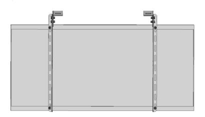
2. Attach the clips to the rails. In each of the mounting holes, use a 5/6 - 18 x 3/4" bolt and flat washer on one side, and a flat washer, lock washer and nut on the other.
