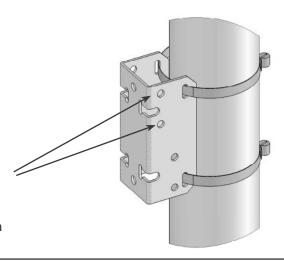
**6.** Tighten the hose clamp screws to 35 inchlbs.
