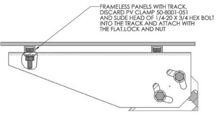
3. Lay the PV Module face-down on a protected flat surface.
