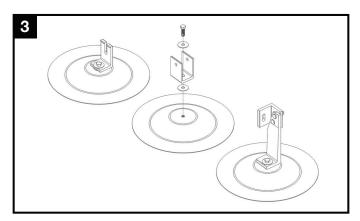
Attach rail mounting bracket with washers and 3/8" hardware torqued to 250 in-lbs (21 ft-lbs). Seal attachment and/or membrane per roofing manufacturer's requirements.
