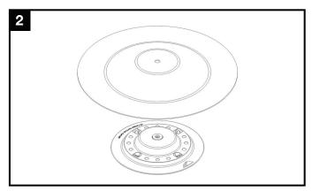
If using a membrane flashing, remove the silicone washer's protective liner prior to attaching the membrane. Thread a bolt into the base to help center the membrane during the welding or adhering process. Ensure membrane flashing is compatible with existing roofing material.
